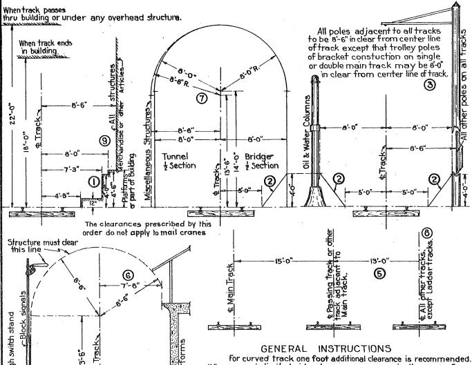
When space is limited side clearance may remain the same for curves not over 12 degrees; for curves over 12 degrees add 1 inch to standard clearances for each degree of curve.
