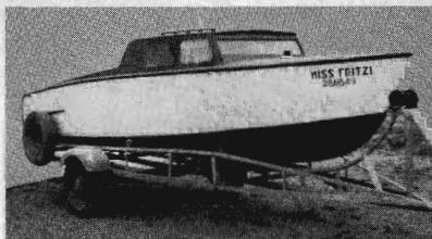
The trailer is built of pipe and angle iron, welded electrically. It is equipped with a one-ton capacity winch which is used to both load and unload *Miss Fritzi*. As a consequence, this 1,000-pound boat can be used anywhere it is possible to drive to.
