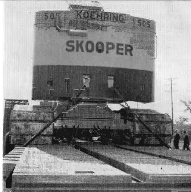
View from rear of flatcar shows two channels in flatcar deck in which winches are positioned to secure inboard tie-down chains. View also shows outboard tie-down chains secured to car sides.
