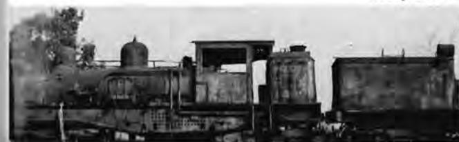
Left: With a unique gearing system this 65-ton Shay, built in Ohio in 1920, once pulled Yosemite Lumber Co. logging trains up grades as steep as 14 per cent.
