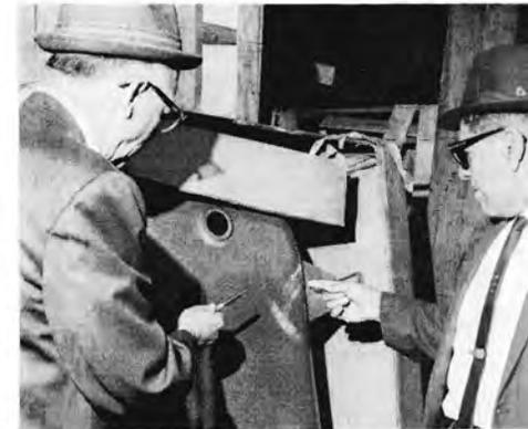
Another example of improper packaging that caused damage to this tub. This has since been corrected by having shipper use a wooden frame to better distribute forces encountered while shipments are in transit.
