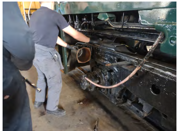
CMO David Elems works to remove a damaged brake cylinder bolt on WP 1503
