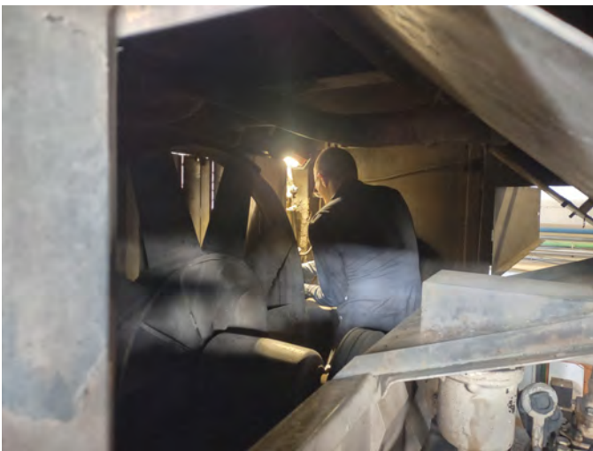
CMO David Elems inspecting, repairing and lubricating cooling shutters on QRR 1100
