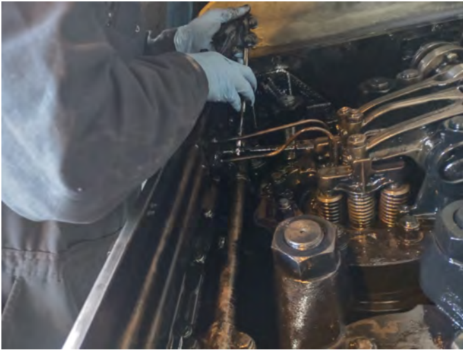
Securing fuel lines after injector cleaning and inspection on SP 2873
