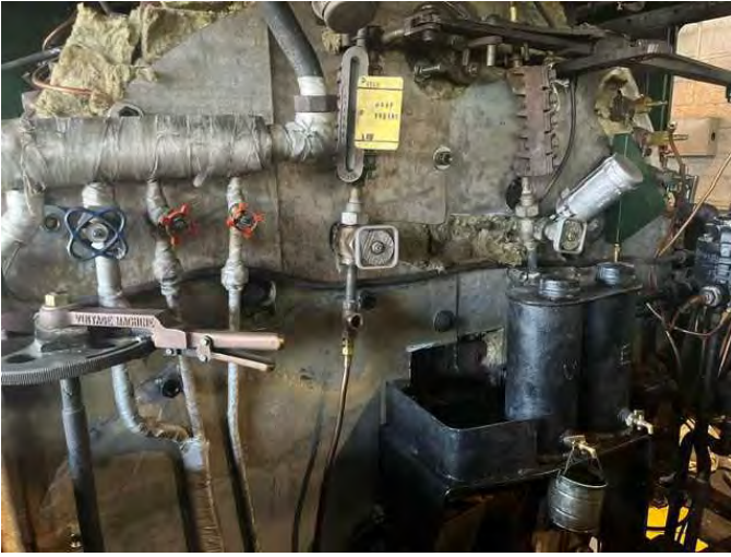
Jacket work completed in the cab. Work done by Roger Stabler and Logan Beers. - Roger Stabler May 2024
