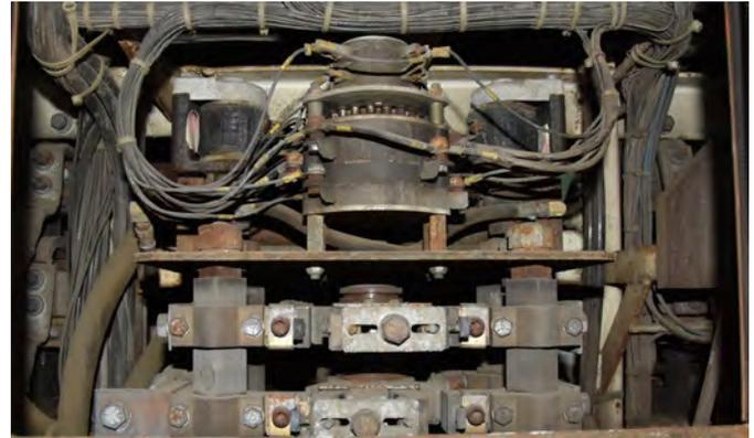
*Cam switch contactor for the traction motors from SP 2873. That is what you hear clicking when you go from power to dynamic brakes. Additional SP 2873 electrical photos are available online at [WPLives.org/trainsheet192](http://WPLives.org/trainsheet192). Photo by Greg Elems*
