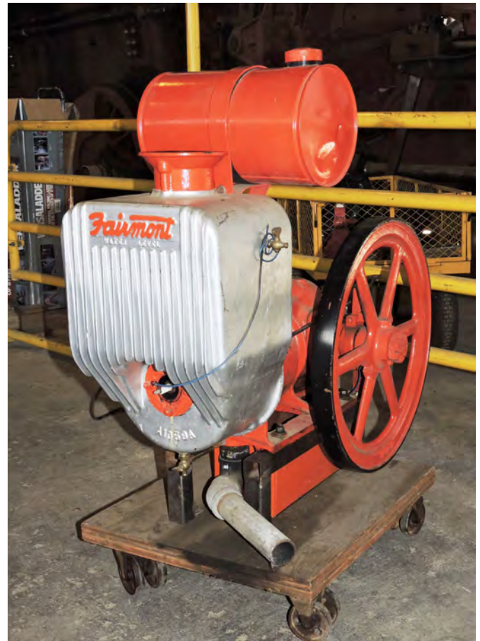
Fairmont motor with double wheels and pulley at the WPRM
