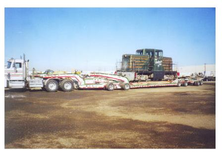
The locomotive arrived Portola at 1 PM on Oct 25, and was unloaded onto our trackage a short time later. We connected short rails from our lead track by the front gate to the rails on the trailer, shoved a flat car up against the locomotive and pulled it off the trailer.
