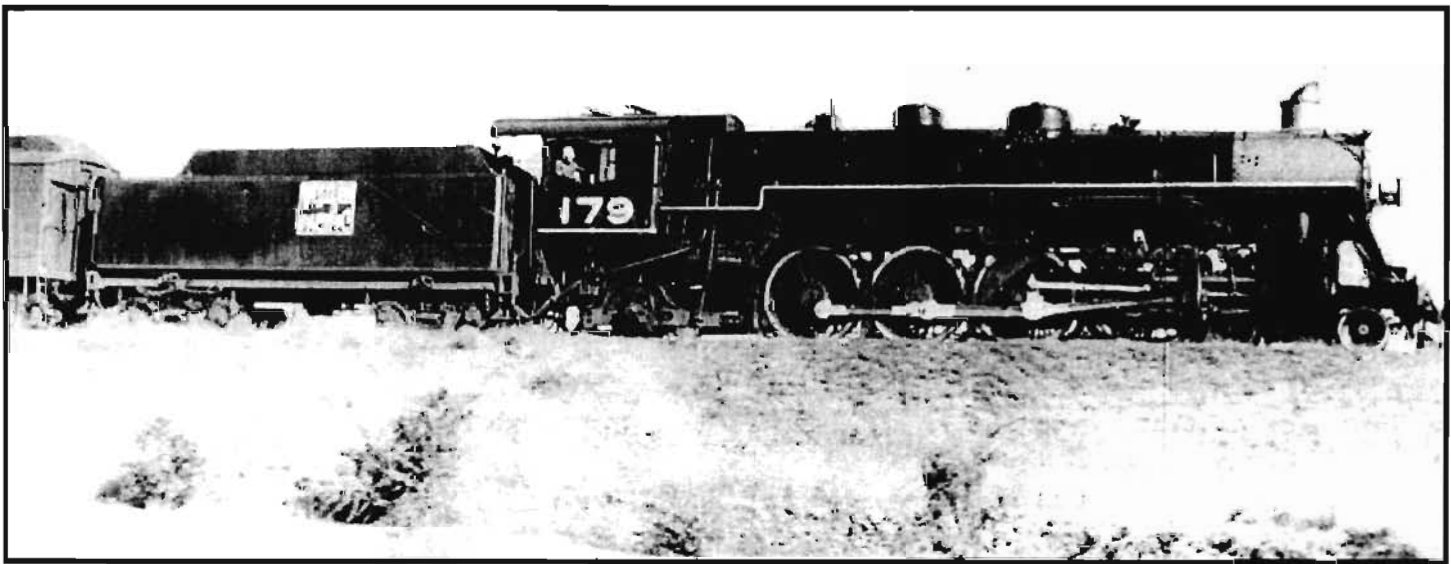
Mountain #179 is pulling into Oroville in the 1940's with heavyweight cars in tow. Note the different smoke deflector attachment on the stack. WP tried a variety of smoke deflection devices on the Mountains, all designed to hopefully keep drifting smoke out of the crews face while running at speed. —Photographer unknown, courtesy Greg Munster
