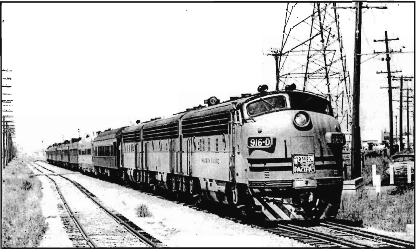
Even though he preferred steam, intrepid steam photographer Bill Pennington would train his medium format camera on a diesel from time to time. Here in the late 1950's he has stopped on film an extra passenger special pulled by an A-B-A set of the Wobbly's F units. 916-D displays her as delivered paint and lettering details as she pulls the special near San Leandro, California. —Bill Pennington, courtesy Greg Munster
