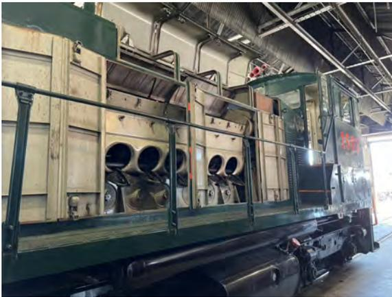
terior of the block, as well as the interior surfaces of the air box. On a two-stroke supercharged diesel engine, the air intake is not just charged for compression, the pressure is also used to clear out the combustion gasses from the power stroke. This process isn't completely smooth, so some of those combustion products end up flowing back into the air box and it makes for quite a mess.
