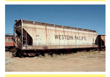
WP 11974 is a center flow hopper and is one of the later ones with the billboard WESTERN PACIFIC on the side. Built in 1975 by American Car Foundry, it is a 4,600 cubic foot capacity, three-compartment car with six individual loading 30" hatches on top. It has a load capacity of 198,000 lbs.
