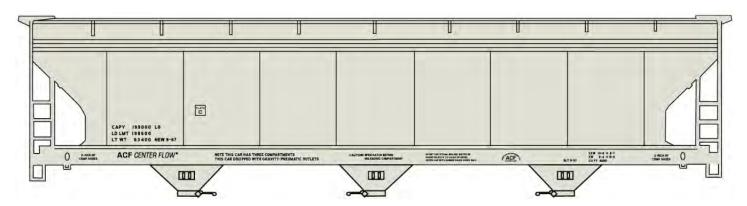
Center flow covered hoppers built by American Car and Foundry are used for shipping all types of dry commodities. Due to their design they are easy to unload using either discharge gates or pneumatic unloading discharge tubes. Several variations of this car were produced over the years in different lengths and with different hatch covers.
