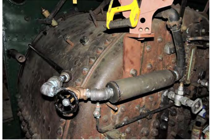
*Fireman's Manifold, body manufactured by Channing Walker. Mike and Roger installed it on the engine with the blower valve and associated piping to the smokebox.*
