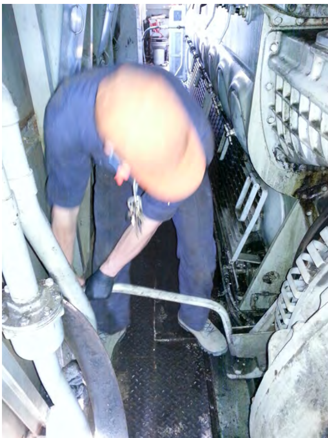
Fritz manually turns over the engine of 917 using the specially designed tool.
