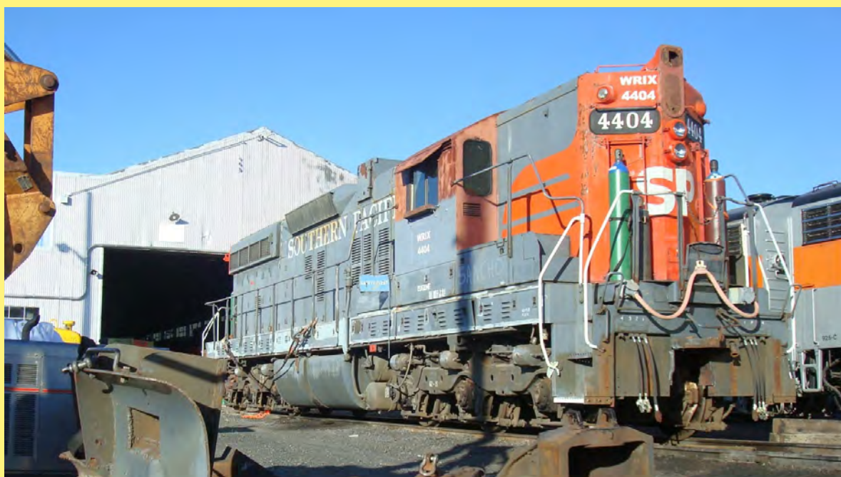
WRIX 4404 (Formerly SP 4404), still in SP's "Bloody Nose" paint, receives facial reconstruction surgery. The locomotive is seen here getting new alignment-control couplers for the move to Western Rail's shops.
