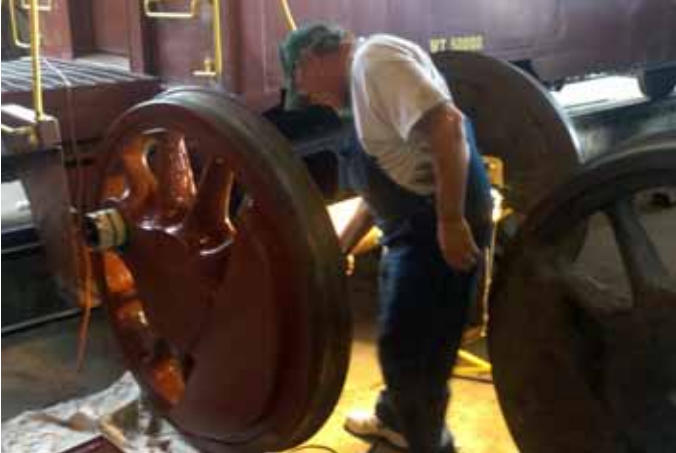
Dick Coudin primers one of the locomotive driver castings. - Chris Allan photo
