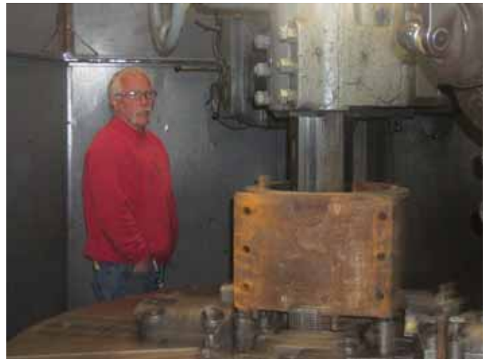
Redman Machine Shop Foreman Mitch Quint oversees the boring of one of the brake cylinders from the 165.
