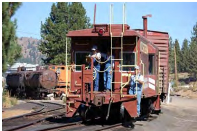
The crew provides protection for the back-up move from the platform of WP caboose 428.
