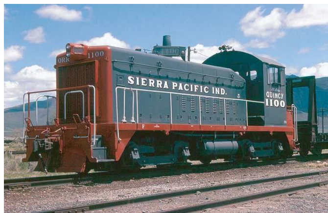
Quincy Railroad 1100 is one of our workhorse engines in Portola. A rare TR6A switcher built by EMD, she served the Quincy for many years. Shown here in Susanville, CA in 1991.
