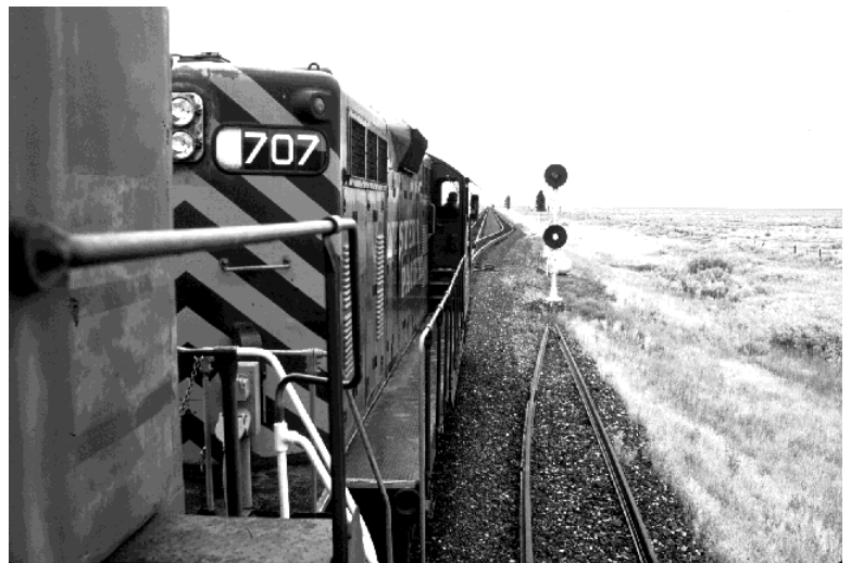
Signal indications confirmed the dispatchers intention to put us in the siding at Hawley and allow faster revenue trains to pass by.
