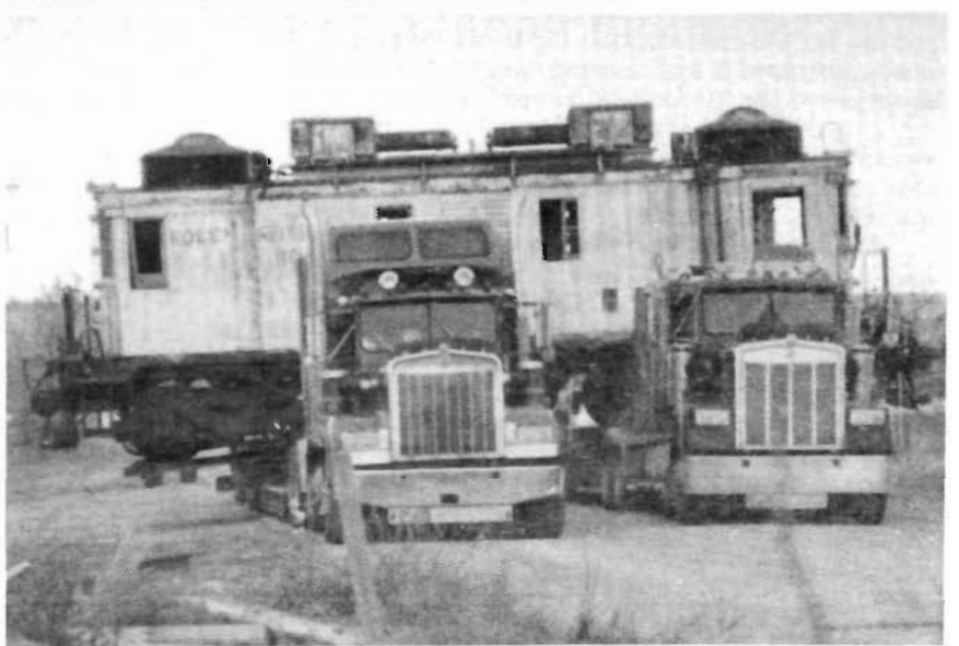
Top photo: The locomotive is being lifted from its long-time resting place in Billings, MT. Lower photo: Following the good advice of the trucking company, Whitewood Transportation, the unit is being moved from its old resting place to the railhead straddling two truck trailers. The two drivers coordinated their speeds using radio communication. Both photos by Norm Holmes.
