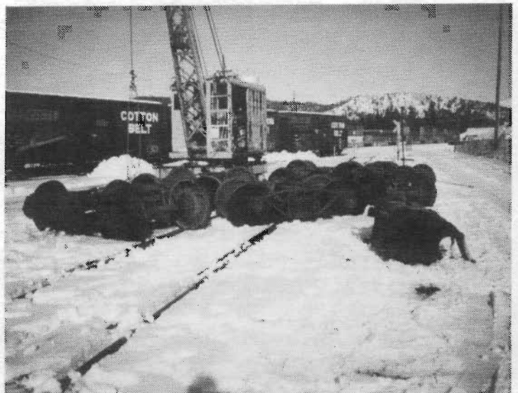
Shown are the arch bar trucks that arrived December 24, 1992 before the BIG snow came. They weigh 6800 pounds each. Norm Holmes did the unloading.
