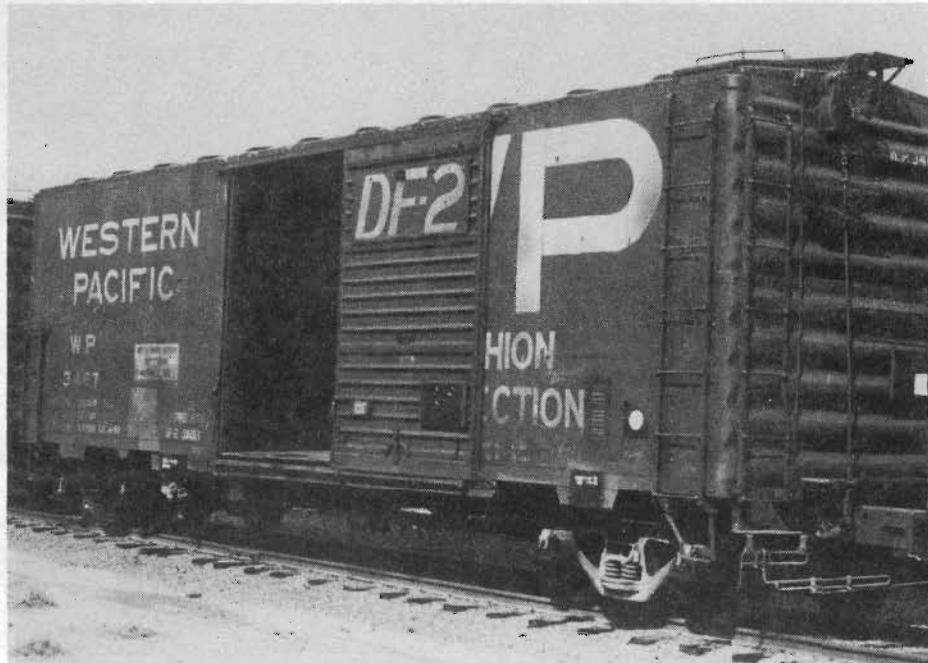
WP 3467 since it has a cushion underframe the end details are as follows, use 1" scale brass wire bent as per diagram, for the cut levers, and the end walk way which all cushion cars have is a set size of 8"X 5'. I made it with Scale Scenics brass Micro-Mesh cut to scale size. Mounted with two 1" brass wires drilled in the end as supports, mesh ACCed in place.
