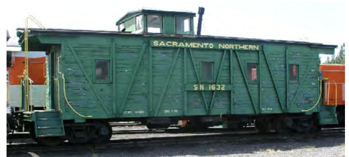
SN 1632 - a Single-sheathed cupola caboose, rebuilt from boxcar 15303 in 1938 by WP
