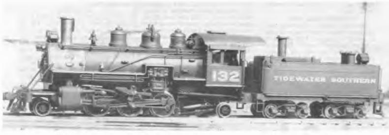
This modified PFM prairie comes pretty close to the prototype TS No. 132. Main differences are in pump, running board positions, and "arch" over pump as supplied with
