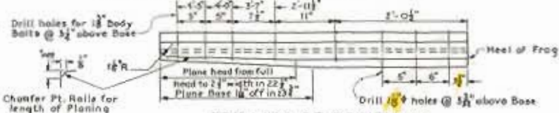
DRILLING OF POINT RAIL
