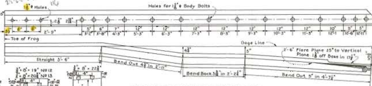
DRILLING & BENDING OF WING RAIL
