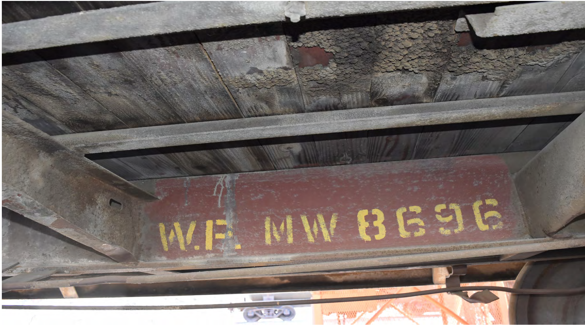
WP 3417 (WPMW 8696) Greg Elems photo Under frame showing one of the car number markings
