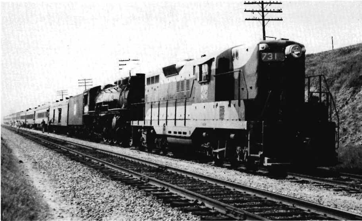
WP GP9 731 (coming to Portola, with sister 725) assists WP 2-8-2 334 (also preserved, at Rio Vista) on a railfan excursion in March of 1956, when the Geep was less than a year old.
