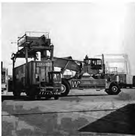
A few minutes from dock side, WP Transport Company's 'piggy-packer' removes container from the flatbed truck onto a waiting flat car.
