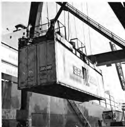
On arrival at the Port of Oakland, giant cranes hoist containers from the container ship onto waiting flatbed trucks for the short trip to the Western Pacific "pig-ramp."
