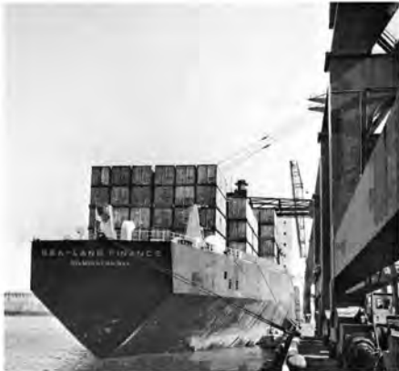
The steam-ship lines and the northern California ports play a vital role in the movement of containers to and from Asia and Europe by ship and across North America via railroad 'landbridge' and 'minibridge.' Fully loaded this class ship will carry 1,096 (35' & 40') containers.
