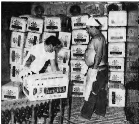
From cooling tube, cartons are rolled into cooled refrigerator car on conveyor.
