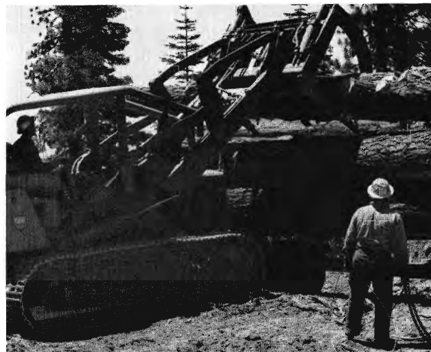
Cat operator maneuvers grapple holding log and deftly drops log in position on log truck dolly. Grapple can be operated similar to person's hand and fingers and a good operator is fascinating to watch.
