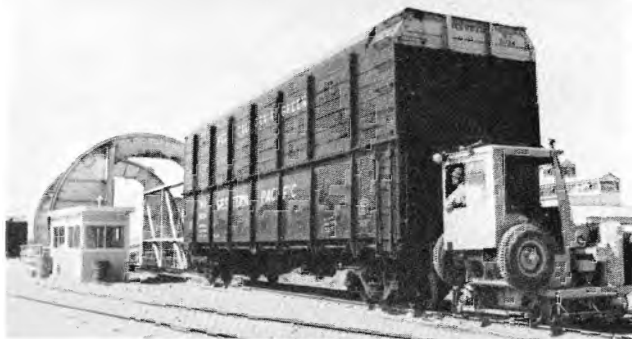
W P chip car being positioned in car turner by Trackmobile at Fibreboard's Antioch plant.
