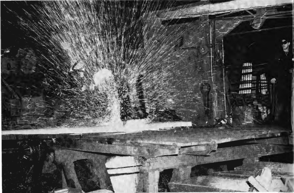
This high-speed, circular "hot" saw cuts the 130-foot-long rail into 39-foot lengths in less than one second. Imperfect ends of the rail strip are cut off and tossed by a man into scrap pans with the aid of long tongs.
