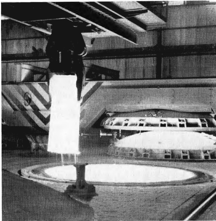
A five-ton ingot is lifted from a soaking pit, a large oven in which the ingot has been heated to the proper temperature before rolling.
