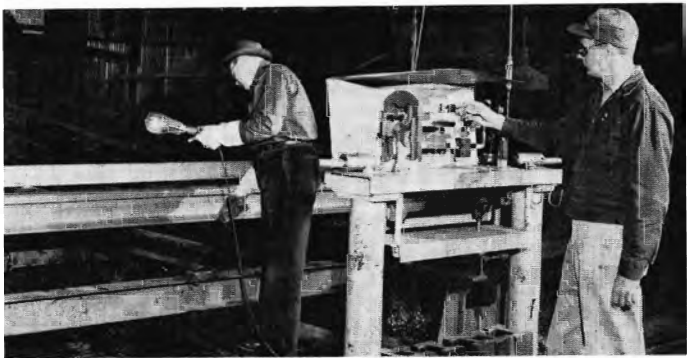
WP Rail Inspector Erich Thomsen checks weight of hot rail as CF&I's Charles Zisk inspects surface of rail. The bright light held by Zisk makes the red-hot rail appear blue, making it easier to see surface imperfections.
