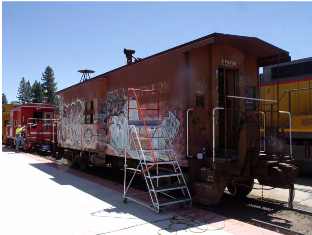
(Above and Below) SP 4706 sits by the loading platform at the west end of the diesel shop in May 2016, as volunteers work on removing many years of graffiti to help new paint adhere better. —Ken Chapin Photos.
