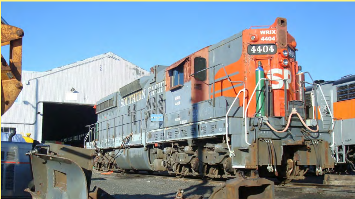
WRIX 4404 (Formerly SP 4404), still in SP's "Bloody Nose" paint, receives facial reconstruction surgery. The locomotive is seen here getting new alignment-control couplers for the move to Western Rail's shops.
