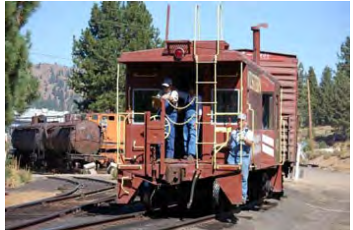
The crew provides protection for the back-up move from the platform of WP caboose 428.
